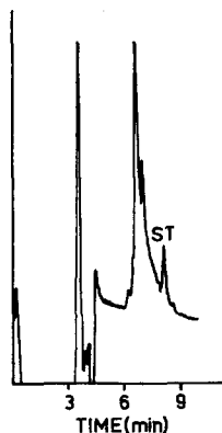
Fig. 7. Chromatogram of a hay sample naturally contaminated with 72 ppb of sterigmatocystin (ST) obtained by HPLC with column switching.
